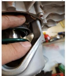
The helix will need to be twisted the proper direction to get the roller in the correct position. The new spring tang will be installed in the same #4 position on the helix, but the spring itself is slightly different torsion value and compressed load. The helix and spring must be turned to that same position when you re-install the helix with the new supplied secondary spring.
