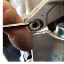
Mark the spring retainer cup and the clutch sheave surface with a marker for re-alignment later.
