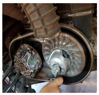
*Figure 1- spread secondary(rear) pulley*
