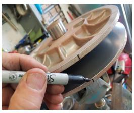
Mark the clutch and take note of both halves and the helix...and position of the roller in the helix for re-assembly. Often, it is best to heat the 3 bolts slightly to release the thread locker before removing.
