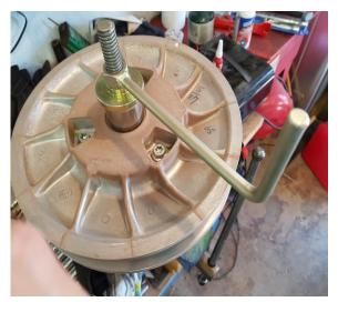
When you assemble the new helix and spring, the helix and pulleys that must be aligned. It is important to have the "roller" of the clutch in the proper slot of the helix and the torsion spring set correctly.
